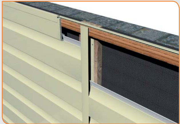
fig 5 Top edge detail showing packing piece and 2-part Universal trim.
