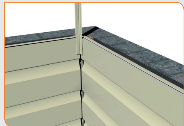
fig 3.2 Showing the male component of 2-part corner trim being applied once cladding is finished
